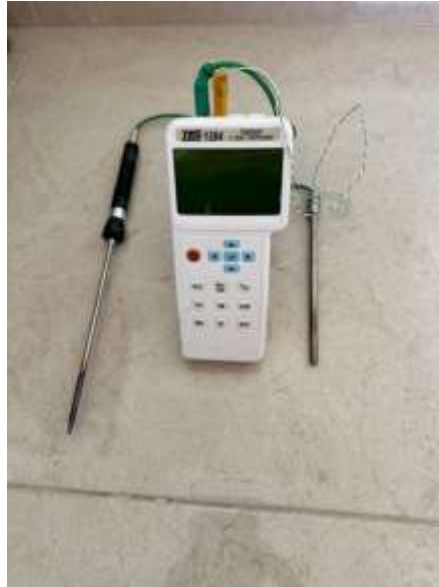
Fig.2. Data Logger and Thermocouples Used for Temperature Measurement
