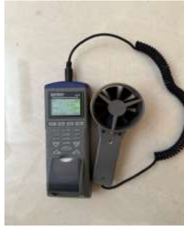
Fig.4. The Air Velocity Meter with A Turbine Wheel Used in the Study
